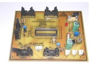
Figure 3. Microcontroller Board
