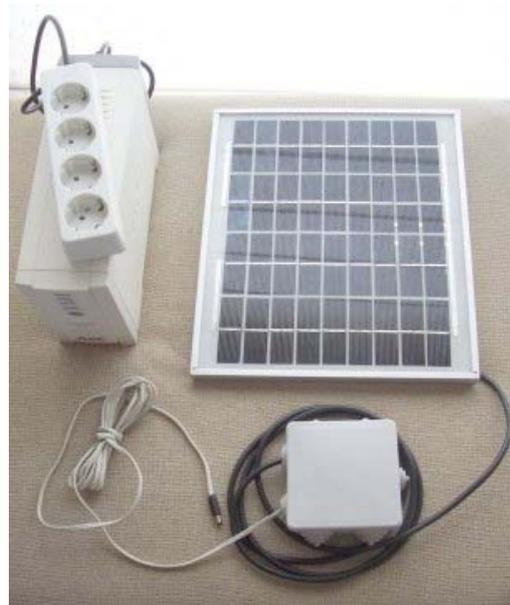
Figure 1. Complete solar kit with panel and AC socket
