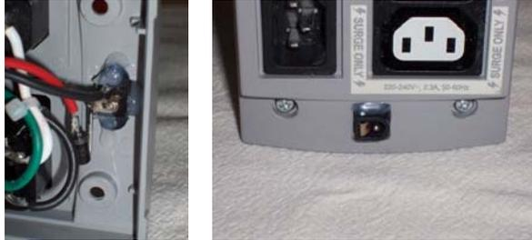
Figure 7. External recharge connector
