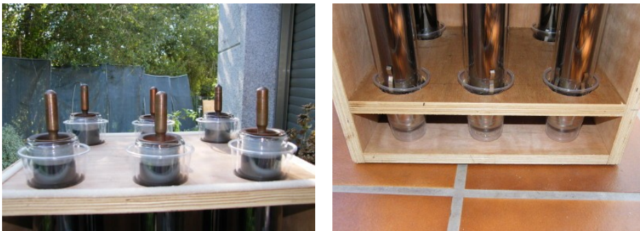
Fig. 8: Vacuum tubes support made of polypropylene cups
