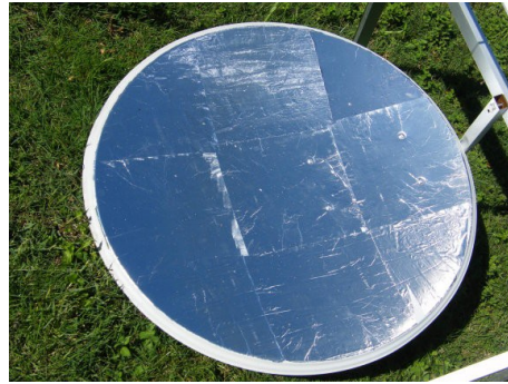
Fig. 7: Different types of reflective cover: polypropylene film (triangular pieces) and aluminium foil (square pieces)
