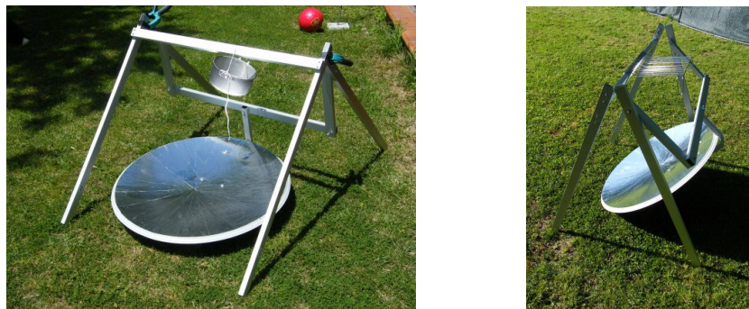
Fig. 6: Finding the focal point of the offset reflector
