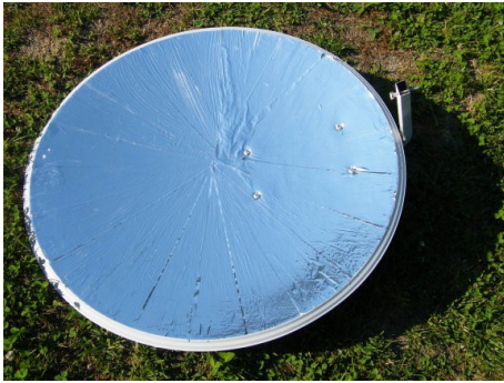
Fig. 7: Different types of reflective cover: polypropylene film (triangular pieces) and aluminium foil (square pieces)
